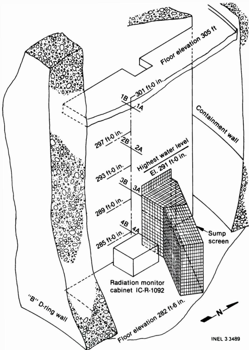
Figure 4. TLD tree analysis beneath core-flood tank.
